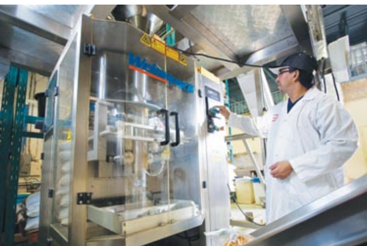
Kumar Seegobin, plant manager, checks the controls on the WeighPack Xpdius Elite 800 bagger that Maywah runs at 60 bags per minute.
