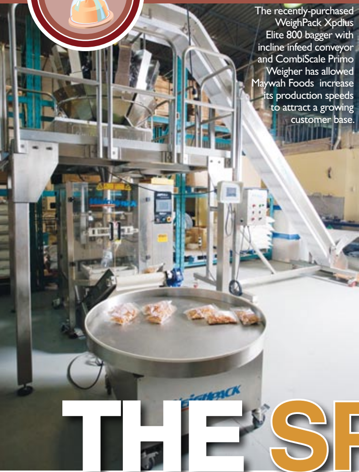
A Baldor washdown-duty motor powers a WeighPack conveyor moving filled bags of product onto a circular accumulator for packaging.
