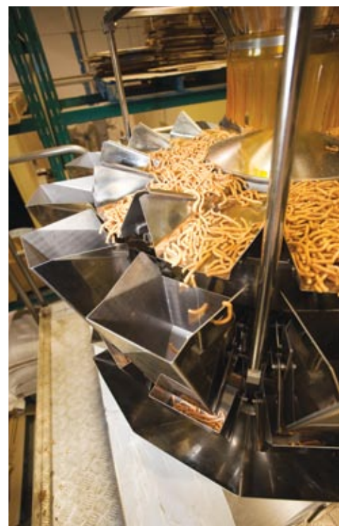
The CombiScale 14-head weigher uses 1.3-liter weighing buckets to distribute precise weights of product into each bag.
